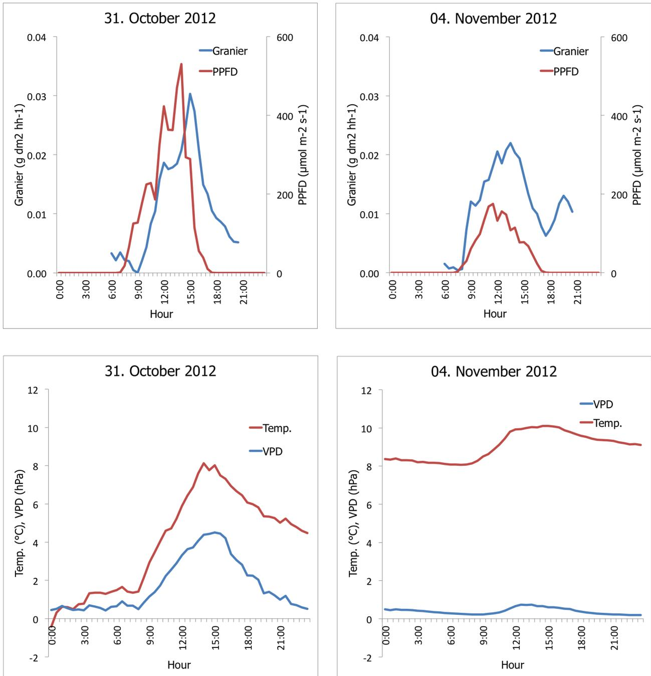
Figure 21.: Measurement of the sap flow density through Granier method for two specific days, in comparison with daily  $ET_c$  trend. In addition meteorological measurements PPFD (Photosynthetically active Photon Flux Density), air temperature and VPD (Vapor Pressure Deficit) are shown.
