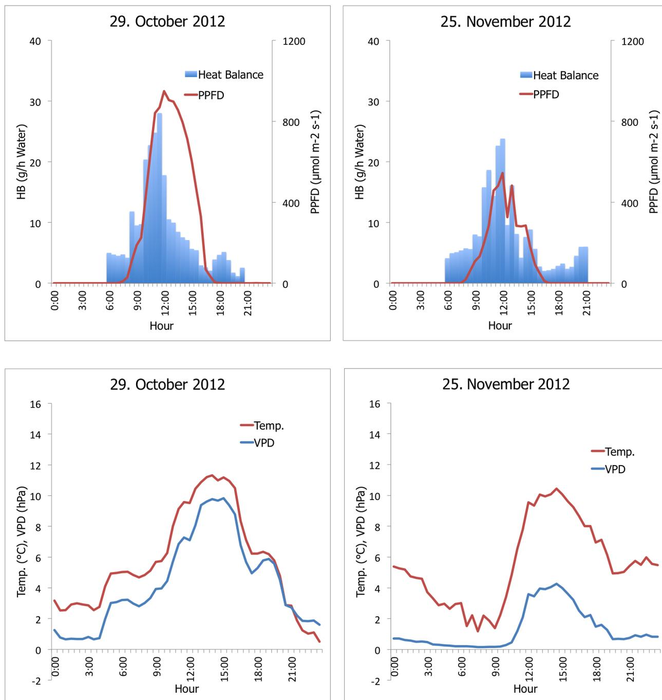
Figure 22.: Measurements of the sap flow rate through Heat Balance sensor on a single branch in comparison with the  $ET_c$  of the whole orchard. The measurements of the flow rate are in g/h. In addition PPFD the air temperature and the VDP for the same day are represented in the figures.
