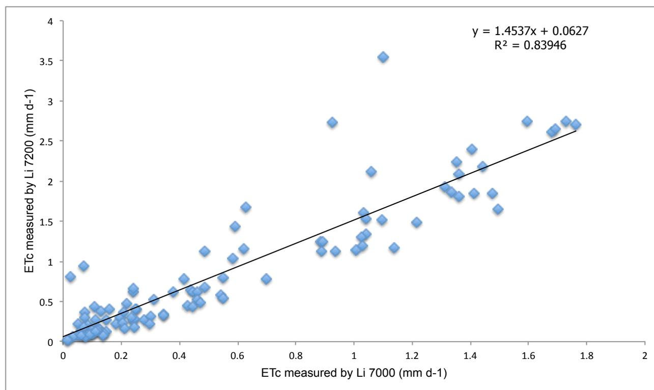
Figure 9.: Data measured from the Li 7000 on the x-axis and the values of the Li 7200 on the y-axis. Regression equation and the  $R^2$  value were displayed in the figure.
