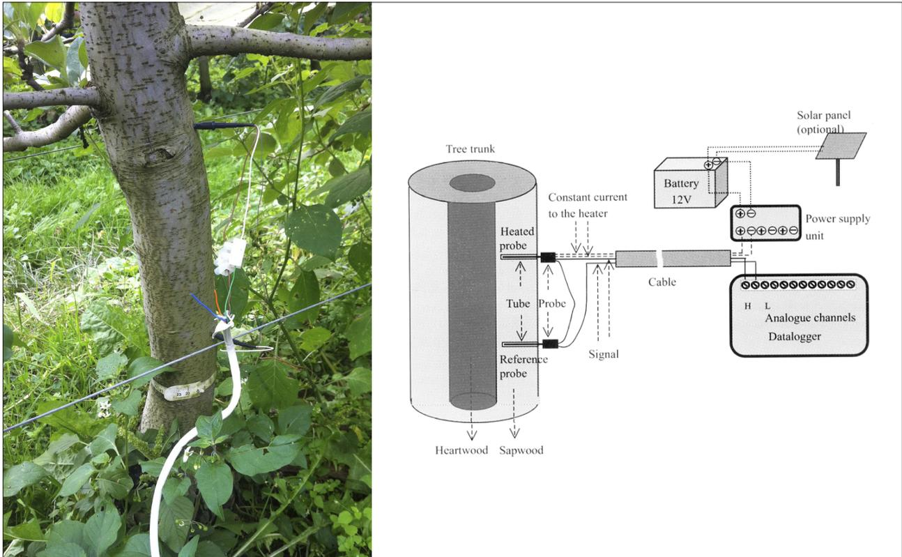
Figure 3: Setting of the Granier sensor on the apple tree E 123. and graphical representation of the experimental set-up of the Thermal Dissipation Probe (TDP) according to Granier (Lu et al., 2004).
