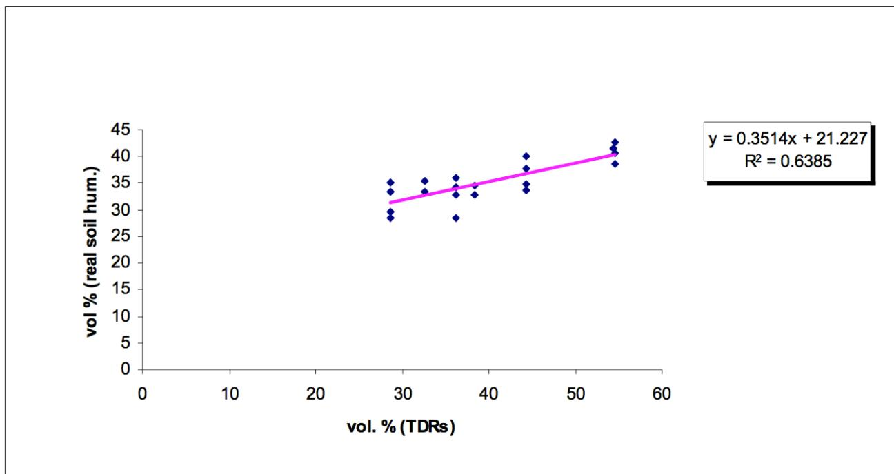
Figure 1: Regression line and regression equation for the calibration of TDRs (Marseiler, 2012)
