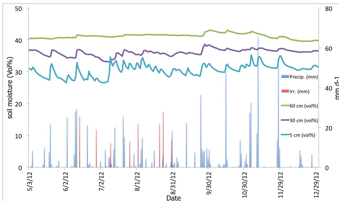
Figure 14.: Daily precipitation and irrigation. Daily average soil moisture content at different depths 5 cm, 30 cm and 60 cm, over the period from May to December 2012. Data until July 15 were taken from Marseiler (2012) and revised.
