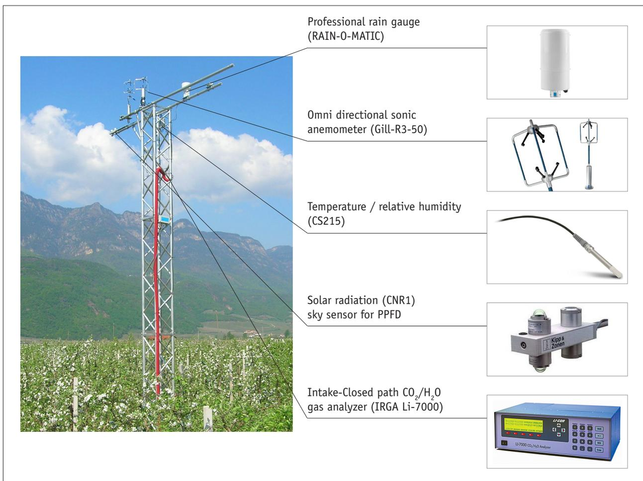
Figure 2: Eddy covariance tower in the study site at Kaltern, South Tyrol, Italy. And the instrument used in the study. (References Picture on Page 45)
