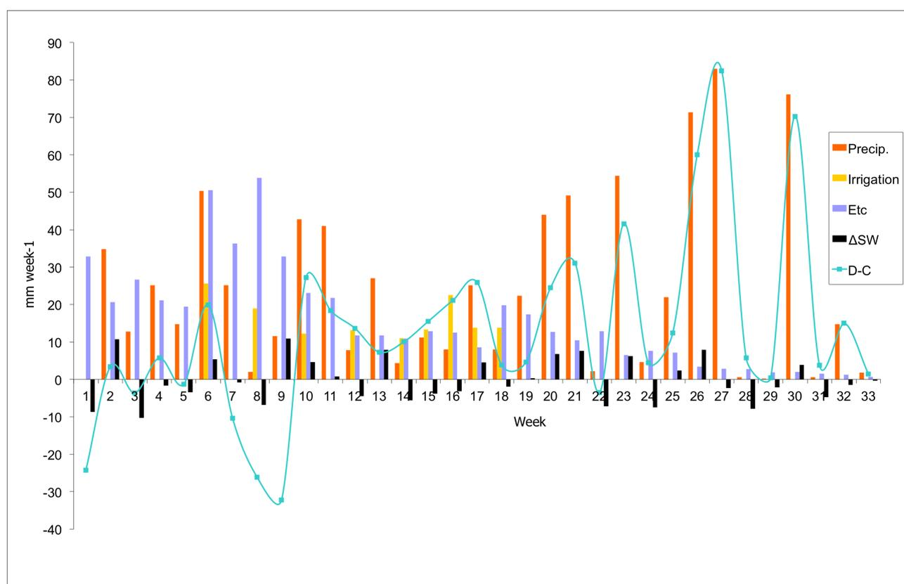
Figure 16.: Water balance of the orchard for 33 weeks from May to December. Irrigation, Precipitation, crop evapotranspiration ( $ET_c$ ), change in soil water storage ( $\Delta SW$ ) and the difference of drainage and capillarity (D-C). Data until July 15 were taken from Marseiler (2012) and revised.
